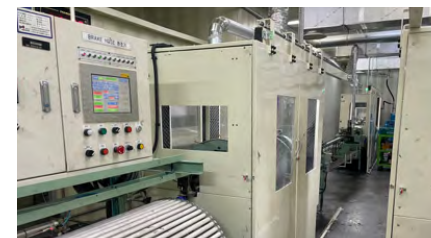
Installing soundproof covers for high-noise processes
